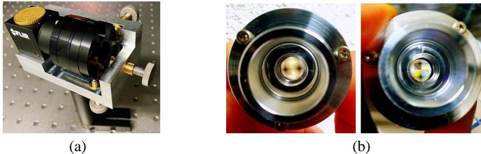
**Figure 1.** (a) Picture of the first realized ASONG prototype including alignment tool; (b) The ASONG optical key components integrated in the prototype.
